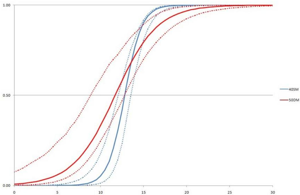
Figure 61. *Mullus barbatus* mean selection curves for the two test gears. Dotted lines indicate confidence limits.
