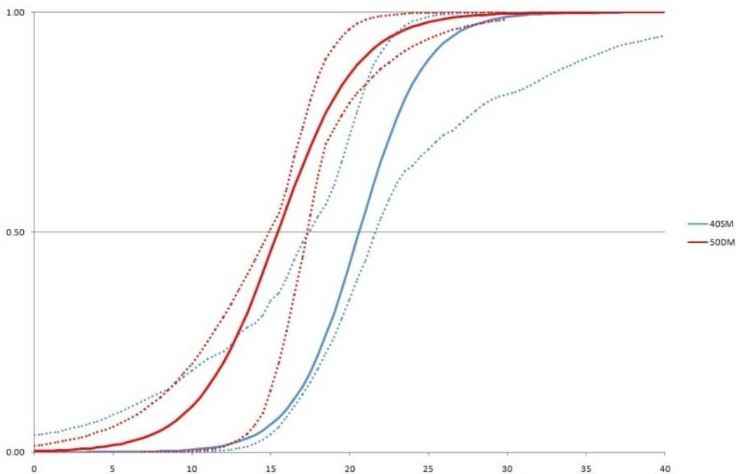
Figure 63. *Parapenaeus longirostris* mean selection curves for the two test gears. Dotted lines indicate confidence limits
