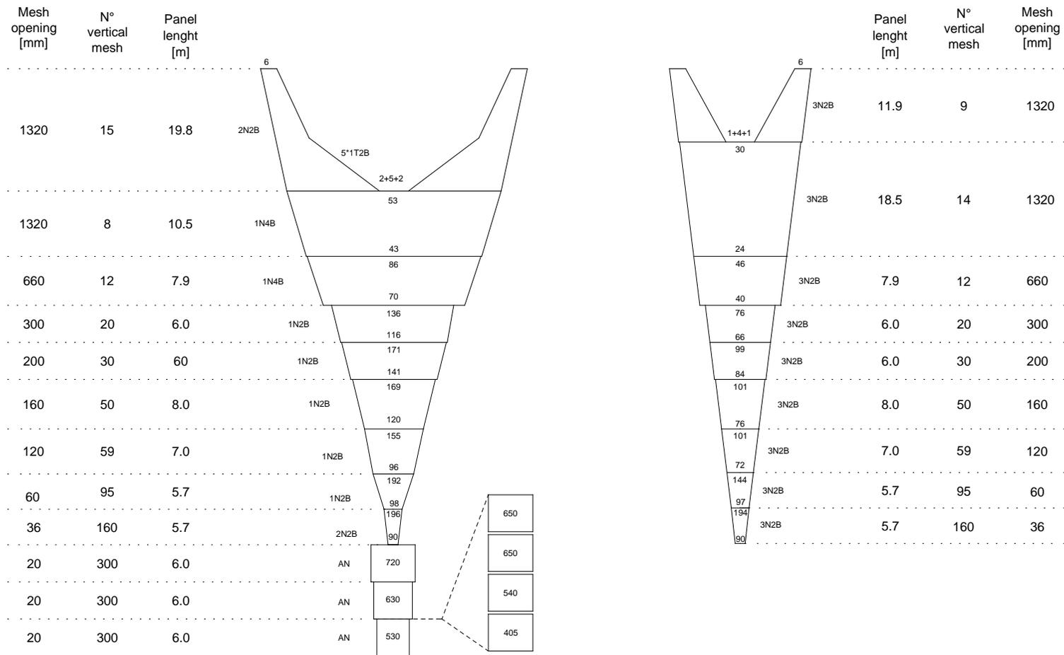
Figure 69. Modified design for the meshing experiment. The four netting sections have been inserted before the last netting piece of the codend.
