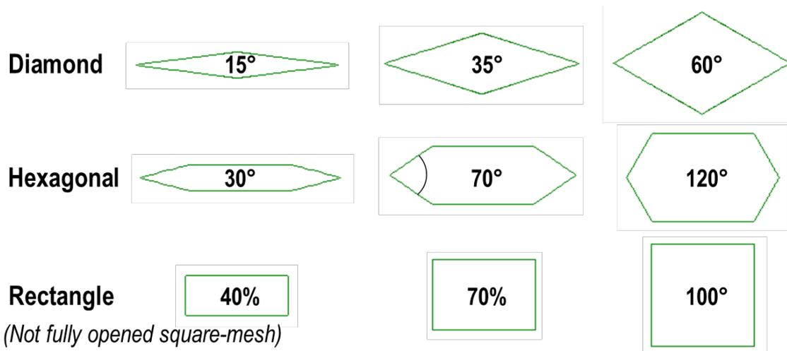
Figure 32. Illustration of the range of the mesh openings investigated both for diamond-, rectangle and hexagonal-meshes for the guideline design of crustacean size-selective mesh.
