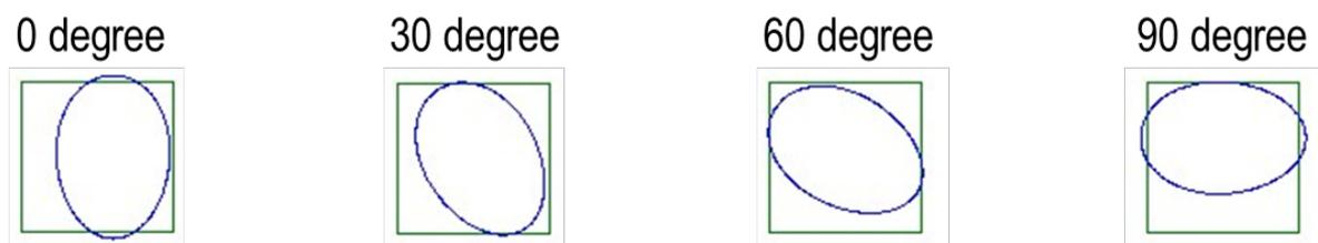
Figure 33. Illustration of potential effect of rotation of the cross section (or attack angle) in a fully opened square-mesh.
