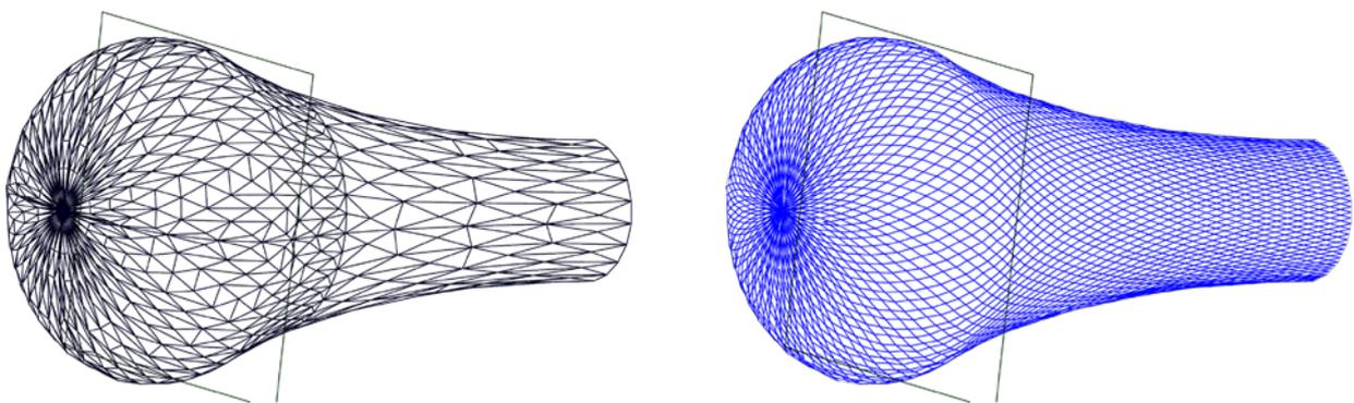
Figure 29. View of the model of codend. The net is split into contiguous triangles in the modelling. On top the triangular element are shown when on the bottom the twines are shown (only 1 on 10 twines is shown). This figure corresponds to p\_d\_ms\_30\_tt\_10\_ma\_800 (see deliverable *D 0.2. Geometry of the codends*) and a catch of 5000 kg.
