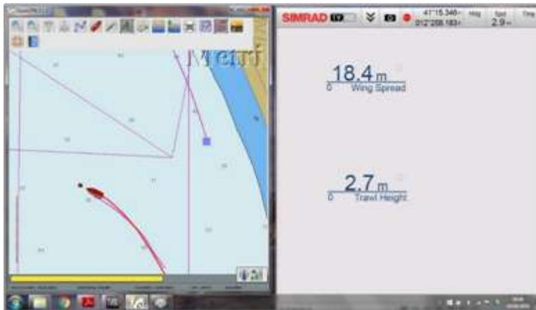
**In each haul, the trawl net was equipped with SIMRAD sensors to monitor the geometry of the net during the towing.**
