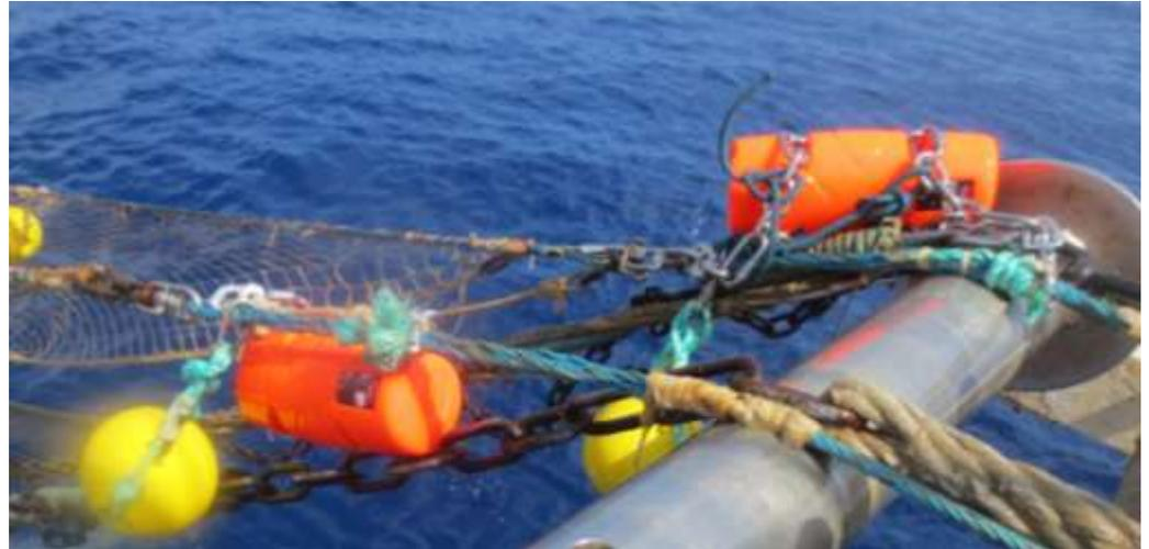
**In addition, a TD probe (DST centi Star:Oddi) was placed on the net to record bottom temperature.**
