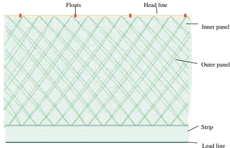
**Scheme of a trammel net equipped with a guarding net (or “Greca” strip).**
